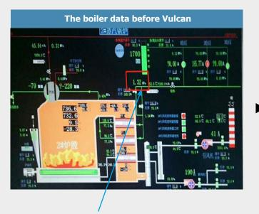
When the operating pressure keeps constant without Vulcan, the pressure on the main water pipe will increase with the time: because the scale will increase, the pressure will also increase.
