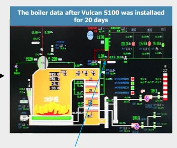
When the operating pressure keeps the same, after 20 days of Vulcan installation, the water supply pipe has been depressurized by 0.12 MPa.
