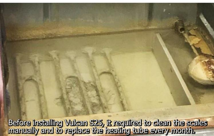
Before installing Vulcan S25, it required to clean the scales manually and to replace the heating tube every month.
