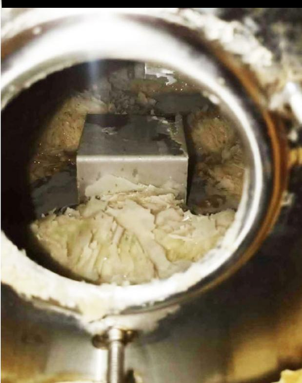
The scale was in flakes and could not be drained out of the steamer's drain hole. To test the effectiveness of the Vulcan system, no cleaning process was carried out before installing the Vulcan S10.
