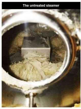
The scale was in flakes and could not be drained out of the steamer's drain hole. To test the effectiveness of the Vulcan system, no cleaning process was carried out before installing the Vulcan S10.
