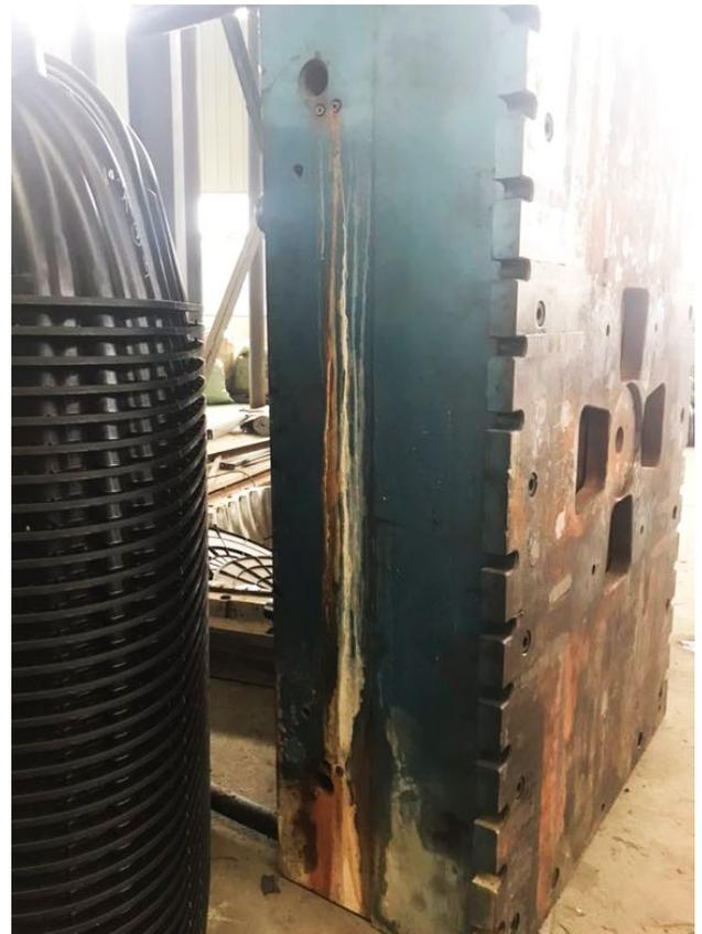
After installing Vulcan S50 for 1 month to treat the mold of septic tank, the scale has already been significantly reduced.
