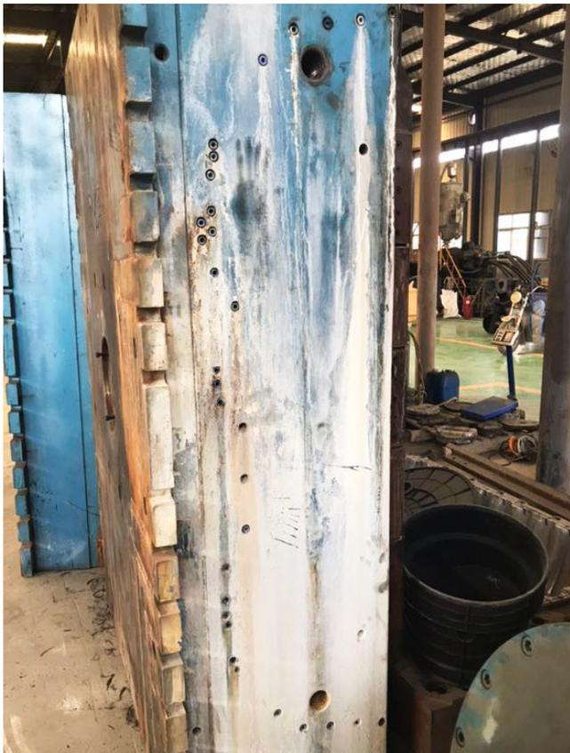
The picture above is the mold of the septic tank without Vulcan treatment. After running for 1 month, it had been scaled badly, and even the small water holes were blocked. Because it was very difficult to clean, it needed to be returned to the original manufacturer for clean up, it greatly affected the production capacity.
