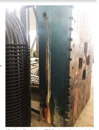
After installing Vulcan S50 for 1 month to treat the mold of septic tank, the scale has already been significantly reduced.
