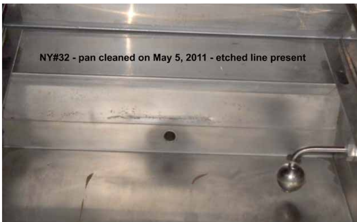
After Vulcan installation - pan area is now completely scale free
