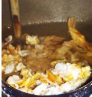
**Pictures 2 & 3.** Scale previously coating the heating element and reservoir sump. (Picture taken from one of the rooms at IBMA hotel)
